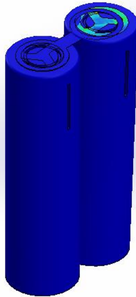
Connector Assembly AA-Horizontal Stress in AA both tab fold-Stress-Stress (MPa)
