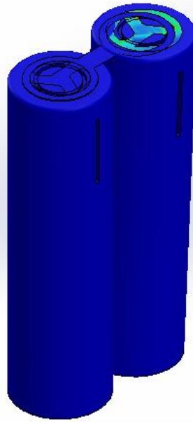
Connector Assembly AA-Horizontal Stress in AA both tab fold-Stress-Stress (ksi)
